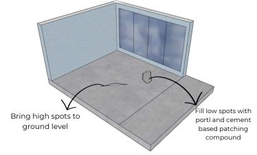
**NOTE:** Gypsum-based patching and leveling compounds are **NOT** acceptable.
