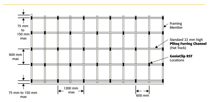
Wall or Ceiling Framing at 400 mm o.c.
